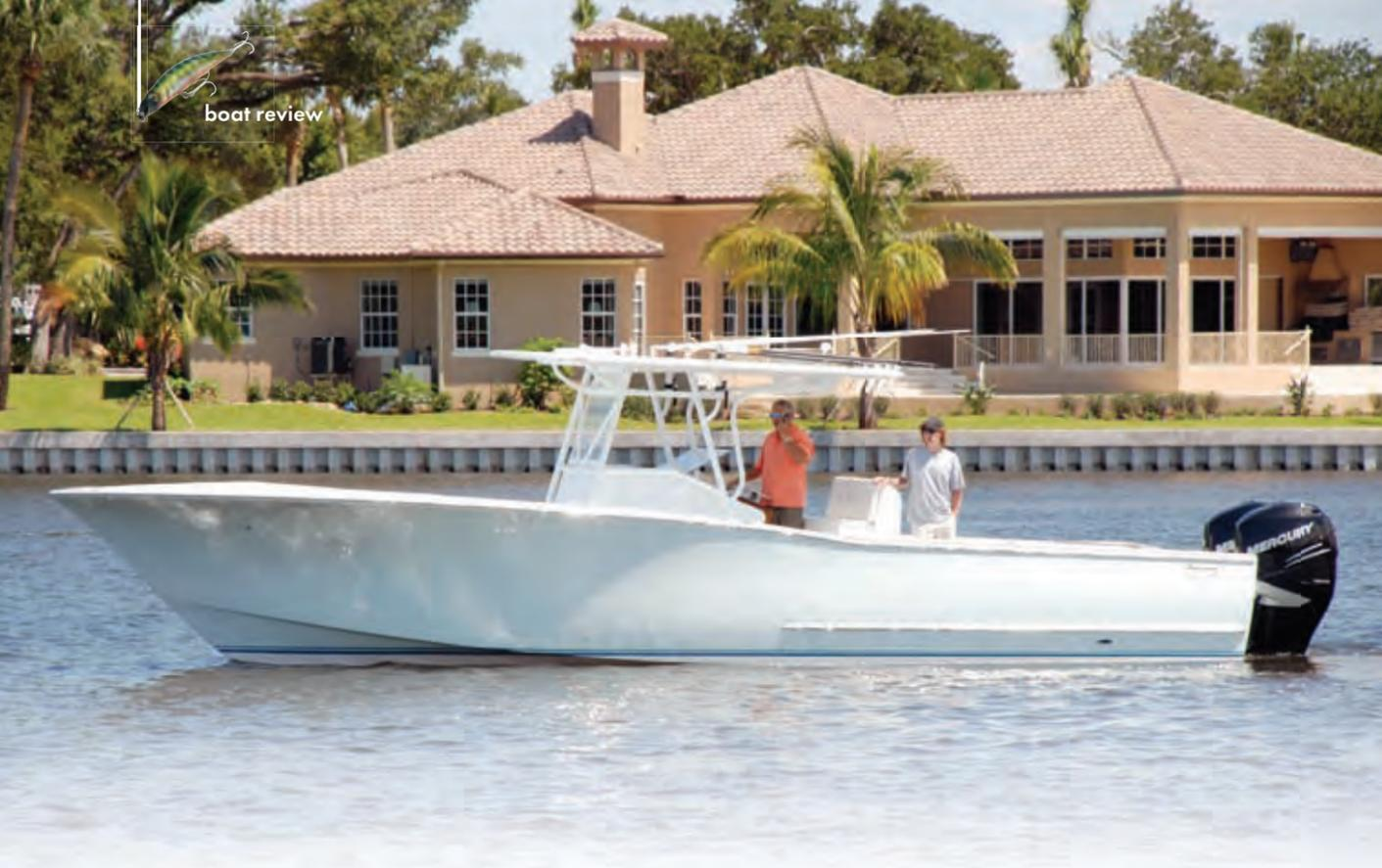
per-smooth, modified-bell/waveform hull design sucking onto the surface of the water. Much like the hull of a large sport fisher, but light and considerably faster.
