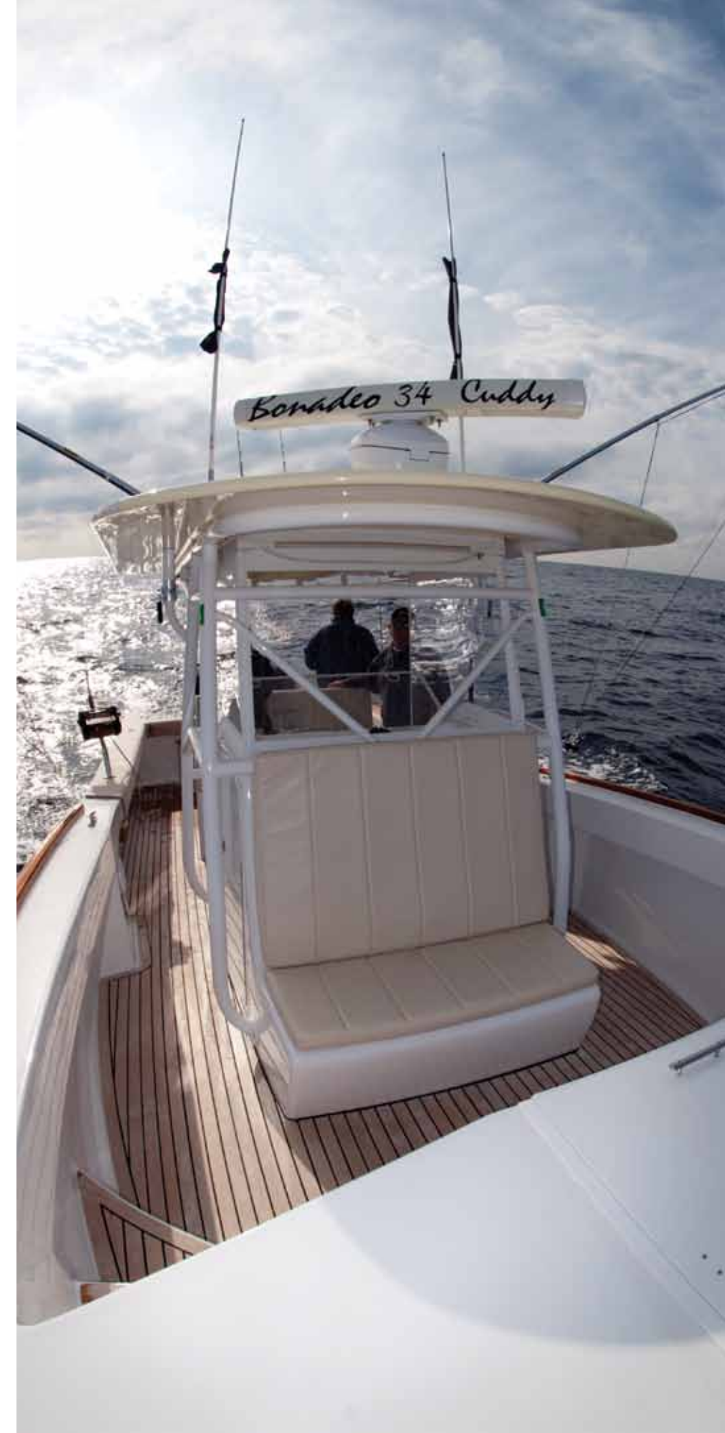
Thick Mahogany toe rail with welded stainless steel rub rails.
